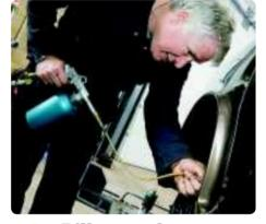
**Pillars and posts 14** With the doors done, move on to the A-, B- and C-posts. Drill access points if necessary and insert the probe upwards and downwards in turn on each post. Slowly withdraw it while spraying. Ian drilled an access hole for the C-post through the rear wheelarch.
