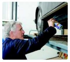
**Rust converter** Once you're confident you've removed any flaky sections, go around and spray rust converter in those areas with surface rust. The converter is a single-pack epoxy - it dispels moisture and, obviously, converts rust. There's no 'build' to it.
