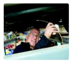
**Probe around** 6 Go around the car and use the spray gun with an extension probe to get wax into all the smaller areas you won't be able to reach when spraying the final coat later.
