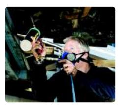
Soft underbelly 16 The last step is to work along the underside of the car, coating the floorpans and other major areas not yet treated. This is where access is key – a ramp will really pay dividends. A pit will also be fine but ensure adequate ventilation is available.
