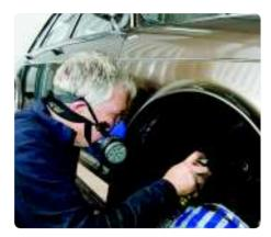
**Fill gaps** 11 Having previously stripe coated the arches and used the extension probe to get into awkward areas, you can now use an aerosol to fill in the remaining gaps. Be sure to shake the can well to achieve the best atomisation and coverage.
