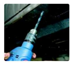
Sill sections 8 If you haven't got access points in the sills, you'll need to create your own. With a car this size and a metre-long probe, lan only needed to create one access hole in the middle of the sill using a 10mm drill bit.
