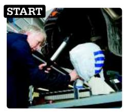
**Front arches** 1 Raise the car and remove the front road wheels. You don't want anything waxy to come into contact with brake calipers or hoses, so use a plastic bag to cover them. If you do get anything on them, wipe off with brake cleaner.
