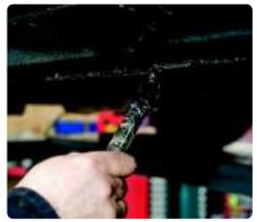
Avoid weak spots 5 On this seam, for example, underseal would fall away from the sharp edge as it dried. This leaves that edge vulnerable. Choosing a product with good hygroscopic qualities means it'll penetrate into seams and absorb moisture.
