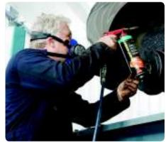
**Complete coverage 15** The main coverage of undercoat is the last thing to be applied. You must have put in cavity wax and stripe coated the seams before this point. Here, lan's applying it using an air-operated Schutz gun - this helps it go on as effectively as possible.
