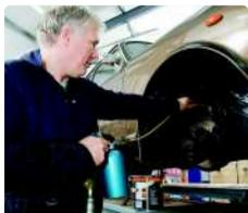
Hard to reach Even if you're not spraying into a cavity as such, applying cavity wax in this way enables you to get into awkward areas and 'fill in' those sections.
