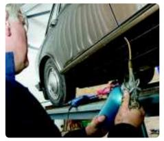
**Smooth action** 9 Insert the probe down the sill in one direction, and draw it out at a smooth pace. Repeat in the other direction to coat the entire sill. Choose a nozzle that gives a fine atomisation - almost like a 'cloud' of wax. This ensures the best coverage.
